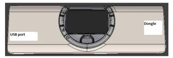
This image shoes the placement of the dongle (USB receptor) and USB on the device viewed from the top. The USB receptor is located in a compartment on the right hand side of the device. The device is delivered with a USB receptor which has been matched to the individual unit. If the USB receptor is lost, a new receptor can be matched to the unit.
